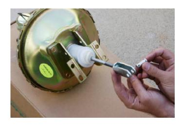
To remove the old master cylinder from the firewall, first suck the brake fluid out of the reservoir with a siphon. Loosen the fittings and disconnect the brake lines from the side of the master cylinder. It's important to cover or cap the lines to avoid contaminants from entering the system. Remove the nuts and washers securing the master cylinder to the firewall. Remove the clevis lock-pin and disengage the master cylinder pushrod at the brake pedal.
