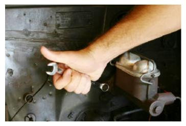
After the fluid has been drained, remove the old master cylinder from the firewall.
